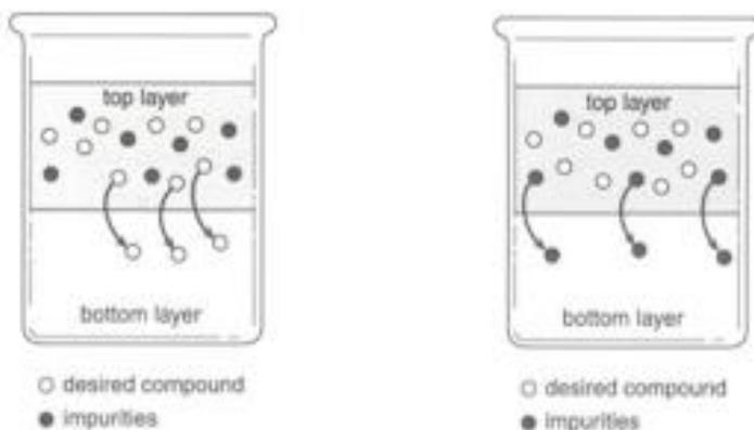
Figure 1 Extraction occurs when the desired compound changes layers, leaving impurities behind
